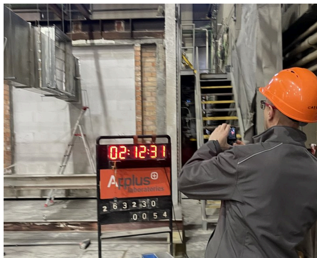
FIRE RESISTANCE TEST OF A GERHMAN DAMPER — ACCREDITED LABORATORY
