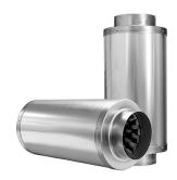
The **Hertz R** is a high-performance round duct silencer developed by GERHMAN for integration between circular ventilation ducts. The construction features an **outer spiral-wound galvanized steel casing** and an **inner perforated sheet steel wall**, ensuring mechanical durability and acoustic performance.
