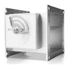
The mechanical CAV-S unit serves to keep the set volume flow constant, independent of inlet pressure and without external energy supply
