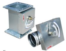
regulators are used for automatic constant air flow control in ventilation installations. They maintain constant air volumes regardless of the changes of static pressure in the ventilation duct. They operate automatically, without any external power supply. Regulation range is from 2 to 12 m/s, operating pressure from 50 to 1000 Pa. Complies with EN 1751 casing air leakage has class C, close blade air leakage has class 0.
